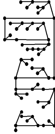
Figure 5.16 Drawing of the tree with n = 57 nodes of Figure 5.13(a) constructed by the Algorithm Arbitrary Spine with A = \sqrt{n} = \sqrt{57} = 7.55 , using Lemma 5.1.
