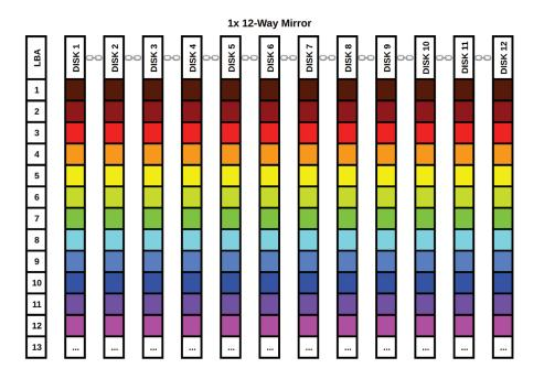
As we can clearly see from the diagram, every single disk in the vdev gets a full copy of our rainbow data. The chainlink icons between the disk labels in the column headers indicate the disks are part of a single vdev. We can lose up to 11 disks in this vdev and still have a complete rainbow. Of course, the data takes up far too much room on the pool, occupying a full 12 LBAs in the data array.
